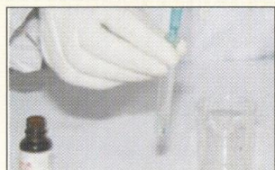
3rd Step: Add 1ml of Reagent-2 in test tube
