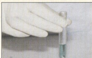
4th Step: Observe change in the color of sample and compare it with test chart
